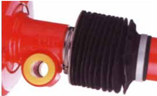
Sewn bellow with a rotating collar at one end fitted to the brake actuator on a railway locomotive
