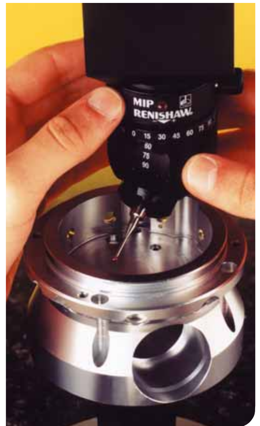
Miniature polyurethane diaphragms are fitted to the probes of high precision measuring equipment
