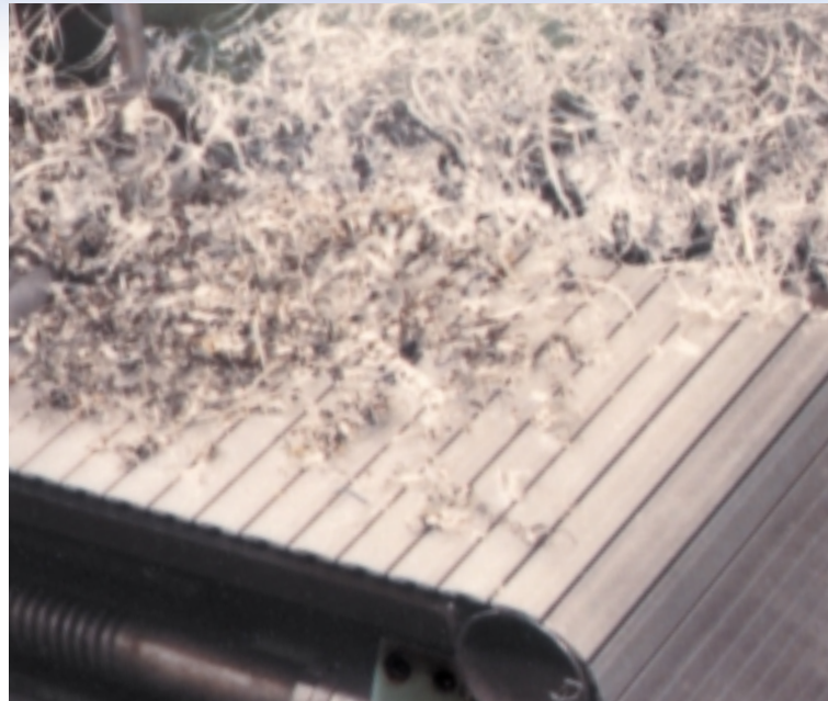
Armoured apron shown in a typical lathe saddle application
